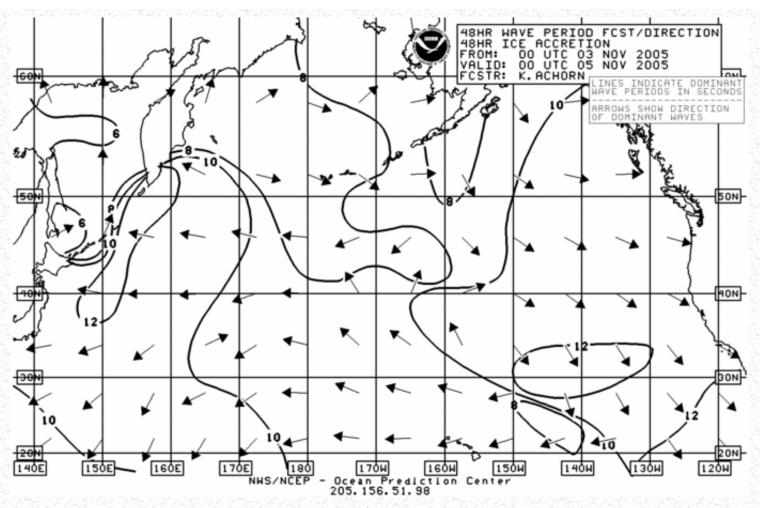
Computer generated chart is generated twice a day from the 00Z and 12Z NCEP computer model runs for 48 hours and once a day from 12Z for 96 hours. The 48-hour and 96-hour graphics are manually edited (00Z Pacific 48-Hour Wave Period Forecast [TIF|GIF| B/W GIF].
