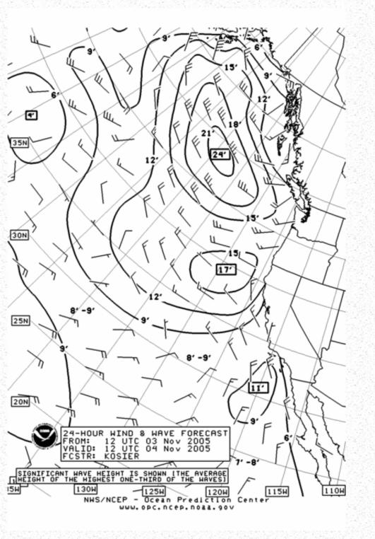
This forecast product depicts 24-hour forecasts of wind (increments of 5 knots) and significant wave heights (isopleths of combined sea and swell in 3 foot intervals). During appropriate weather conditions such as "North Wall" episodes
